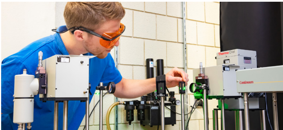
One of many spectrometers that are regularly used in the physics department. Here, Andrew is observing the sample compartment of the time-resolved flash photolysis spectrometer which measures the light-induced absorption changes of photoactive proteins.
