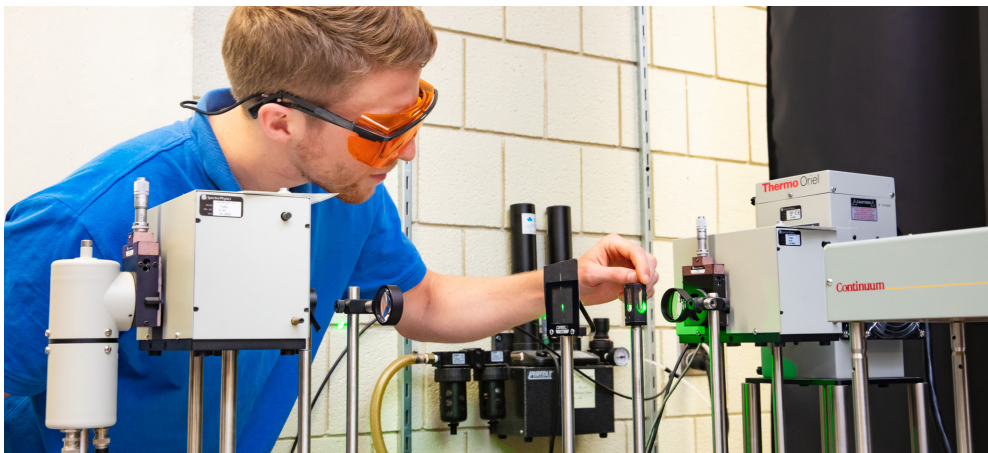
One of many spectrometers that are regularly used in the physics department. Here, PhD candidate Andrew Harris is observing the sample compartment of the time-resolved flash photolysis spectrometer which measures the light-induced absorption changes of photoactive proteins.
